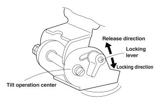
Move the locking lever on the mechanism section of the main unit's bottom panel in the counterclockwise (release) direction, tilt the viewfinder to the desired angle, and move the lever in the locking direction to lock it at this angle.
